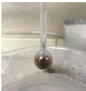
Figure 2: Intercalation in liquid ammonia.
