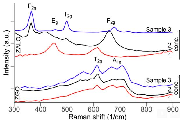
Figure 2: Raman spectra of undoped ZGO and ZALO. The reactant concentration highly affects the peak positions in the ZALO samples.
