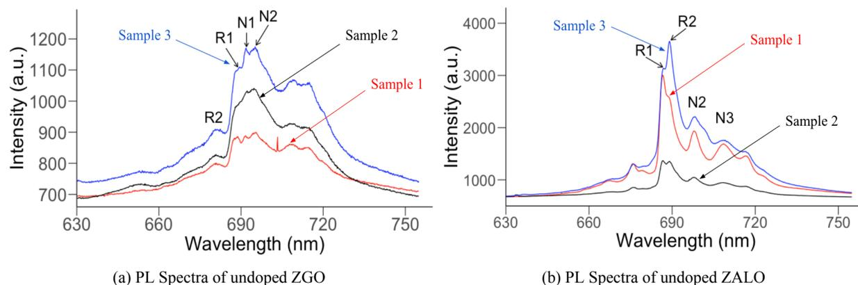
Figure 3: (Photoluminescence) PL Spectra of undoped ZGO and ZALO at room temperature under the excitation of 532 nm.  $\text{Cr}^{3+}$  dopant is found in both samples from the emission peak around 690 nm. The sharp PL peaks are from the zero phonon lines of differently perturbed  $\text{Cr}^{3+}$  ions. The reactant concentration affects the peak intensity and peak ratio as well.
