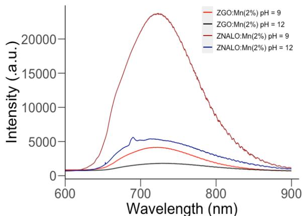
Figure 4: PL Spectra of 2% Mn doped ZGO and ZALO samples with basic pH values under the excitation of 457 nm. The huge and broad PL emission peak at the infrared range is only observed in the basic pH samples.
