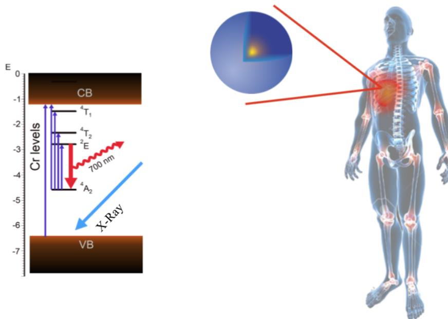
Figure 1: The figure on the left is the energy diagram of  $ZGO:Cr^{3+}$ . Doped spinel oxides can be excited by X-ray photons and emit visible or infrared light. Such emission can be used to trigger phototherapy anywhere inside the body.
