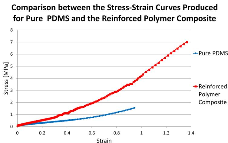
**Figure 2:** The composite demonstrates similar ductility to the PDMS up until the PDMS breaks at about a 1.0 strain ratio, following that the PE properties dominate.
