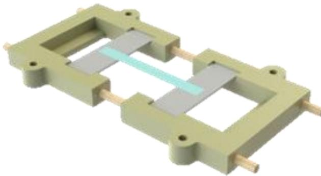
**Figure 1:** This stretching device was custom made for this project using SolidWorks.
