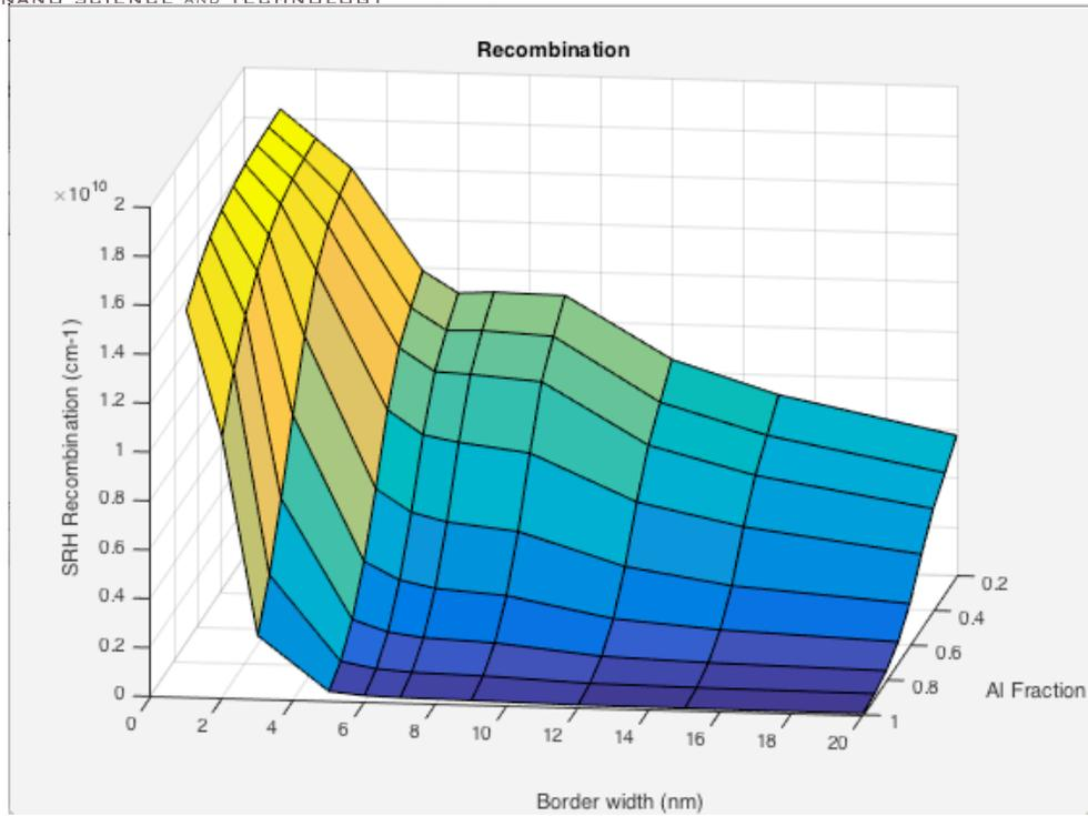
Figure 2. Recombination versus border width and Al fraction
