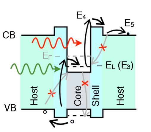
Figure 1. Energy bandgap of CSUN upconversion model
