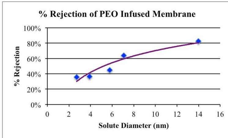
**Figure 2:** One of the charts that is the result of the T.O.C. tests conducted where percent rejection is shown for the various solute diameters for the PEO infused membrane, where the PEO was 9% of the overall polymer mass
