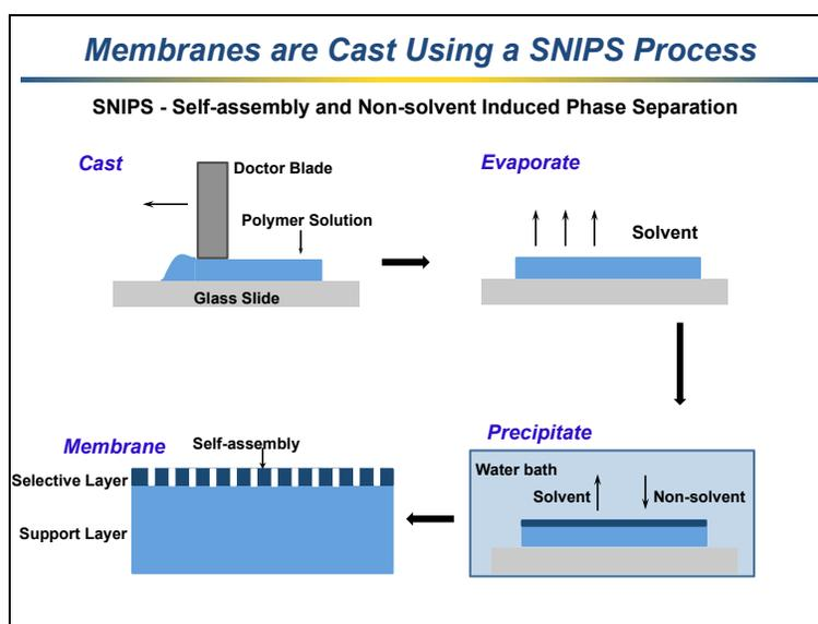
**Figure 1:** A detailed diagram depicting the step-by-step procedure of the SNIPS (non-solvent induced phase separation) method, which is used to easily cast membranes from polymer solutions using a doctor blade, a chemical fume hood, and a solvent solution such as isopropyl alcohol (IPA)
