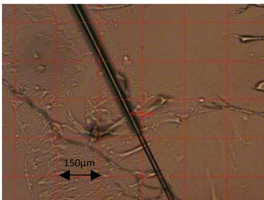
Fiber at rate of  $0.05\text{mm/s} \sim (1.09\mu\text{m})$
