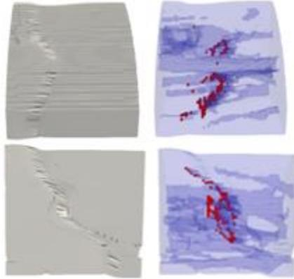
*Figure 4 Finite element model output displaying the failed elements within a yielding sample.*
