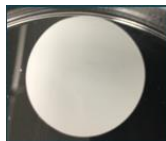
A) Excess Isopropyl Alcohol Bath for 15 minutes to kinetically trap the nanostructure
