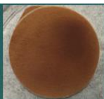
B) 3 hour bath in 10 mL of 1.0M 1,6 diamino-hexane to functionalize the membrane
