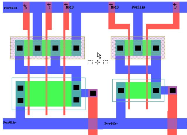
Figure 1. Sample of a 2input and 3input NAND logic gate for implementation in adiabatic circuits with 2 power clocks (PwrClk+ and PwrClk-)
