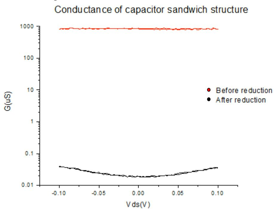
Figure 3. Effect of a reducing environment on the conductance of the capacitor structures. An increase in the conductance implies a reduction to the Nickel Oxide layer at each of the Nickel electrodes.
