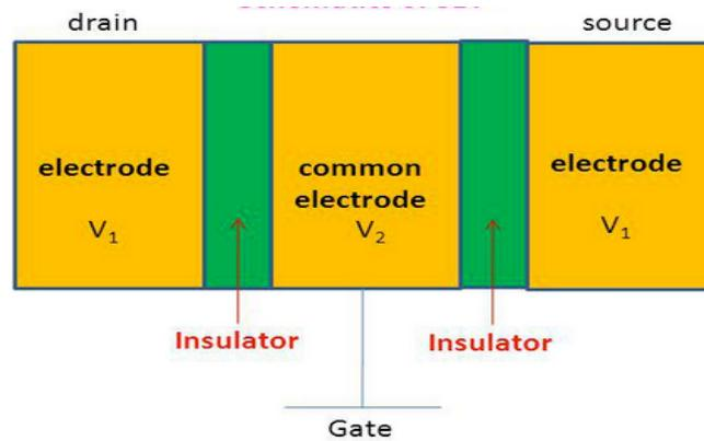
Figure 2. Single Electron Transistor (SET) layout.<sup>1</sup>
