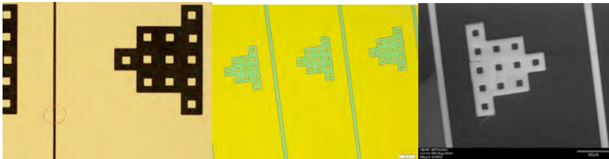
Figure 2: Various steps of the fabrication process. Microscopic images from the left: the photolithography mask (50x), a sample after dielectric deposition and photolithography (20x), and a SEM image of the same sample after 12 minutes of reactive-ion etching and removal of photoresist (50x).
