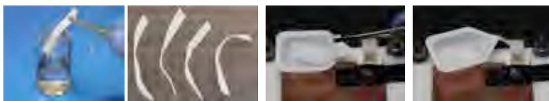
Fig. 2. Process of preparing samples for extractive SAW analysis. a) Saturation of a paper strip. b) Paper strips drying. c) Rewetting in solvent. d) Placement on SAW device.
