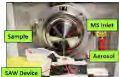
Fig. 1. SAW MS Apparatus.
