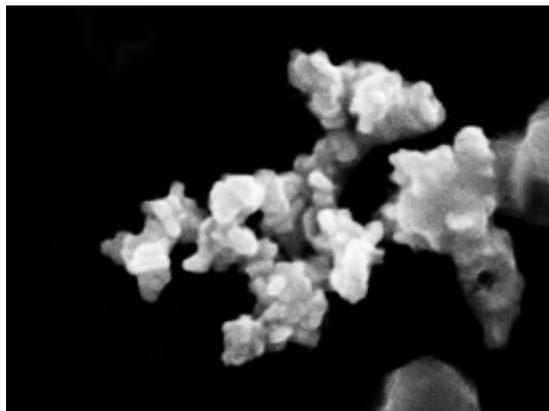
**Figure 1: Lead Sulphide image from SEM**
