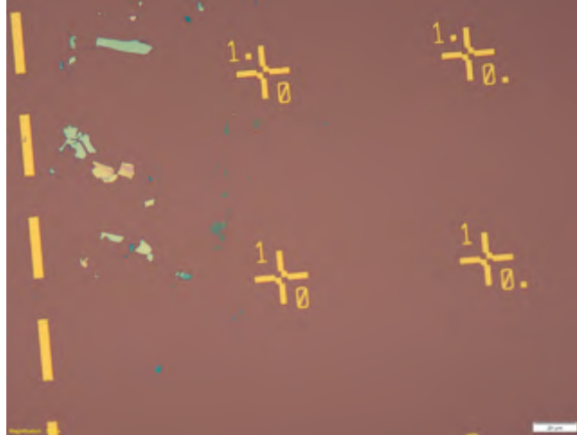
Fig.2: Substrate with MoS 2 flakes on it
