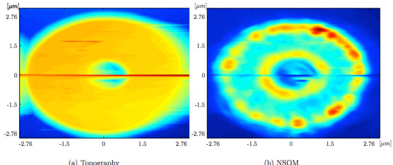
The image on the left is a topographical view of an optical cavity, and the right image is an NSOM image of the same sample, showing where the intensity of the photoexcitation signal was greatest. The colors are relative heights in (a) and relative intensity in (b), where red is high and blue is low.
