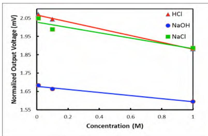
**Fig. 2** Linear fit to show how the output voltage varies linearly with the concentration of the chemical. Further experiments are necessary to prove the linear trend line. All data points are for .1644 THz where there was adequate separation between the different concentration transmission signals.
