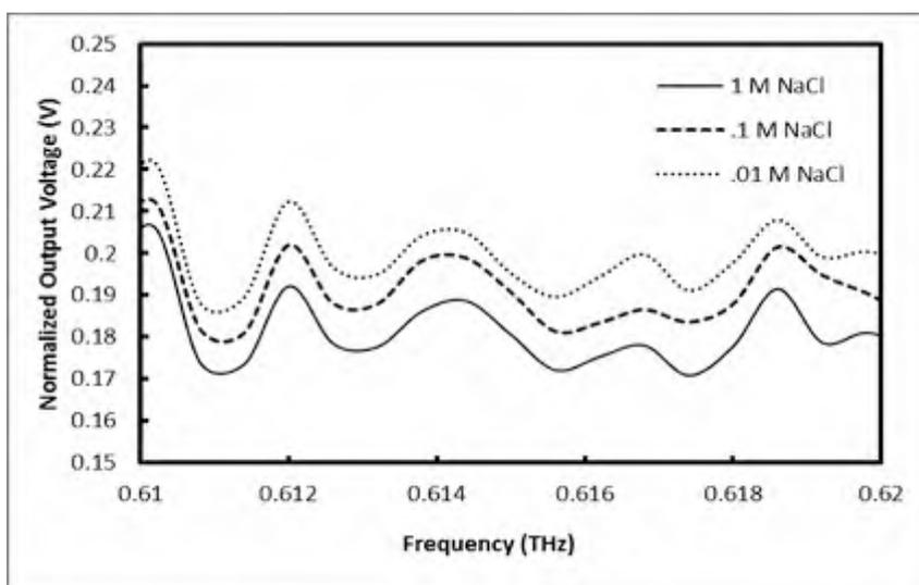
**Fig. 2** The zoomed in normalized output data for different concentrations of aqueous NaCl measured using THz-FDS. The more concentrated solutions absorb more terahertz waves because they form intermolecular interactions with the water molecules that are stronger than hydrogen bonds.
