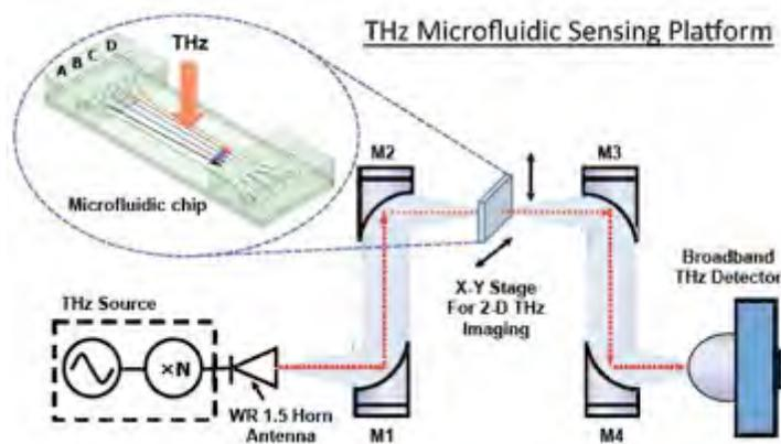
**Fig. 1** The terahertz microfluidic sensing platform includes a terahertz source which is reflected through a series of curved mirrors to gather the waves and create a focal point on the microfluidic device and the detector for increased accuracy and sensitivity.
