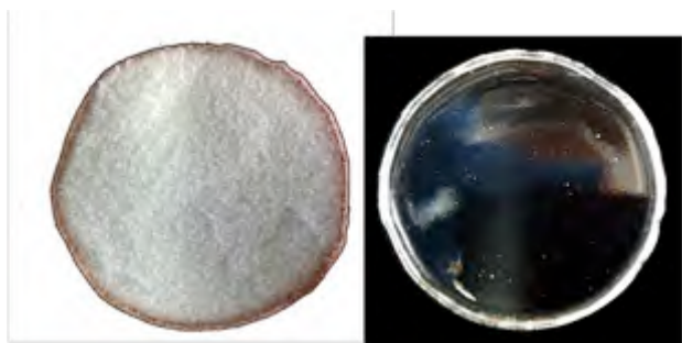
Figure 1. Fabrication of a polystyrene slide. (a) Solid polystyrene powder in mold before melting. (b) Cooled slide removed from mold. (c) Finished and sanded slide with pinholes.
