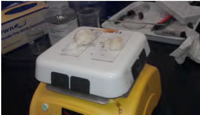
Fig. 2. Samples being heated on a hot plate to evaporate benzyl-alcohol.
