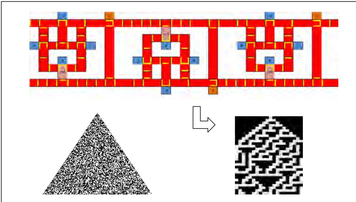
**Figure 1. Top:** 3 cells of the nanomagnetic circuit that performs the logic for Rule 30. **Left:** the theoretical pattern produced by Rule 30. **Right:** the pattern produced by simulating the circuit expanded to 20 cells and extracting the values from the “out” magnets at every time step (matches theoretical pattern, proving that the system works).
