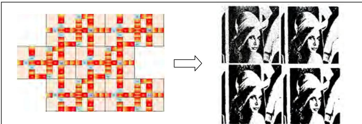
**Figure 2. Left:** 6 cells of the NML circuit that performs the noise reduction illustrated in the **right hand** image. The top left girl is the original noisy image, and its pixels serve as the input to the CA system. The top right, is the output after 4 time steps, bottom left is the out after 8 time steps, and finally, bottom right, 12 time steps – by this time the noise has been fully removed.
