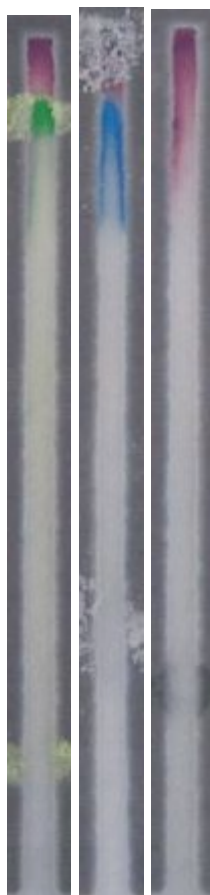
Figure 3. Cobalt Thiocyanate test positive result for amodiaquine, left; positive result for chloroquine, center; negative result, right.
