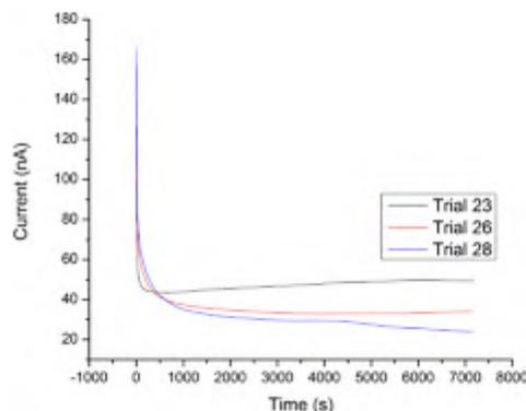
**Figure 3.** Wagner polarization test over 2 hours at 1 V
