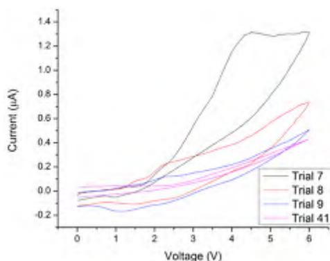
**Figure 2.** *I-V* measurement of graphene/SPE device from 0 to 6 V (double sweep)
