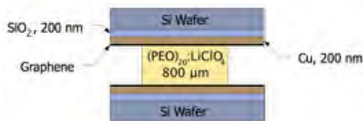
**Figure 1.** Side view diagram of graphene/SPE device
