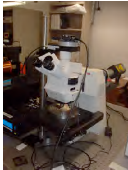
Figure 2: Modified Microscope MOKE
