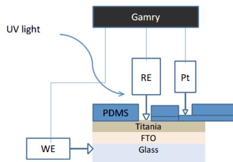
Figure 1: The 3-electrode system
