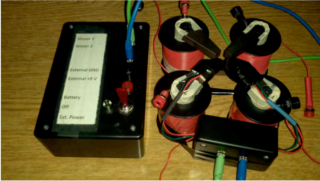
Figure 4: Completed electromagnet and control circuit
