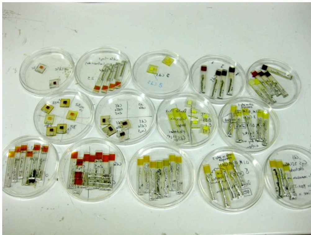
Solar cells: FTO glass electrodes with TiO 2 and CdS/CdSe/ZnS/Cu 2 S layers
