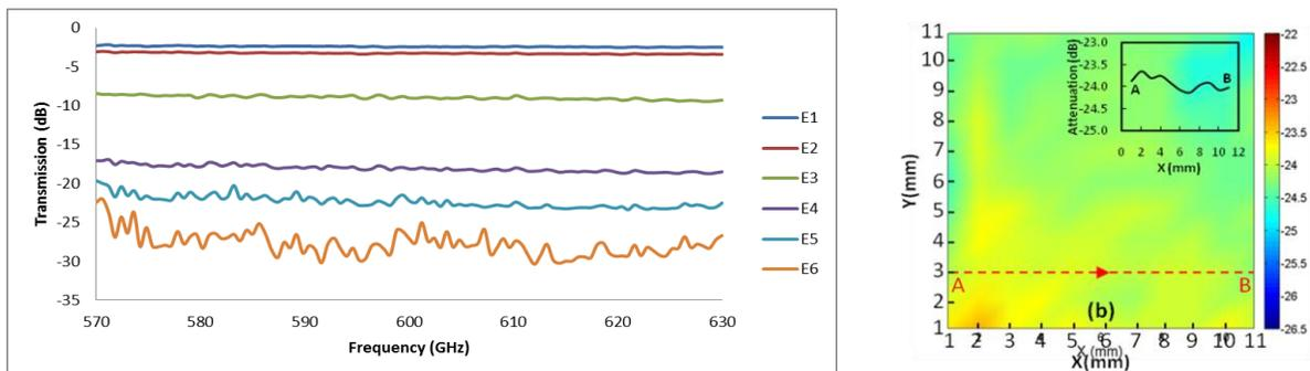
Fig 2a. Graph showing attenuation which increases with increasing loading from E1 to E6 samples.
