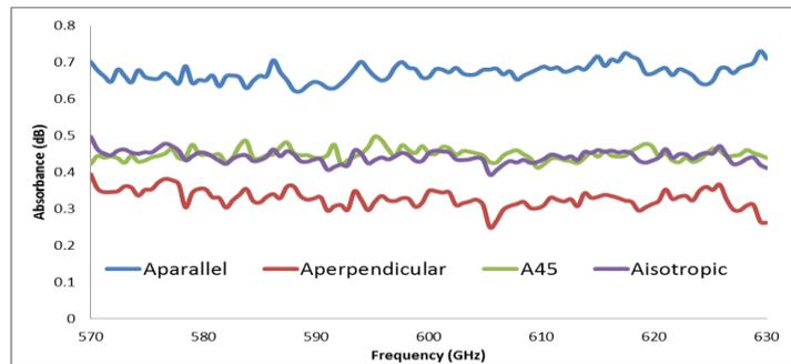
Fig 2b. Absorbance curves for polarizer at various angles of polarization
