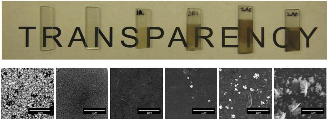
Photographs and SEM images of FTO slides coated with TiO<sub>2</sub> (5 μm thick) and reduced graphene oxide (1-4 layers) and deposited Ag clusters using UV irradiation at different times. (a) FTO, (b) FTO/TiO<sub>2</sub>, (c) FTO/TiO<sub>2</sub>/RGO, (d) FTO/TiO<sub>2</sub>/RGO/Ag (1 min irradiation), (e) FTO/TiO<sub>2</sub>/RGO/Ag (5 min irradiation), and (f) FTO/TiO<sub>2</sub>/RGO/Ag (10 min irradiation). Note the growth of Ag clusters during UV irradiation in panels d-f
